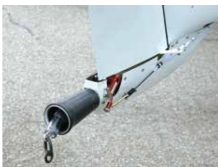
Cable stop plate unit with guillotine and rubber funnel in MCR
