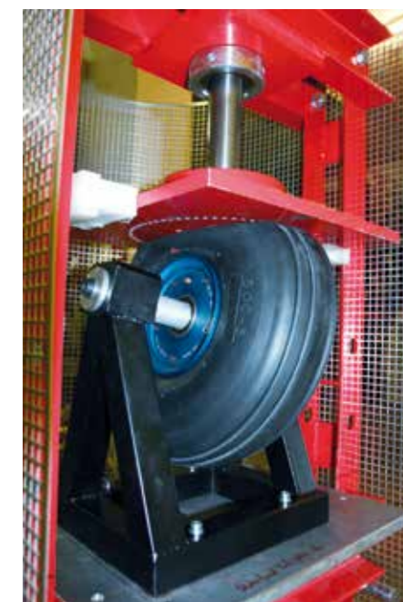
Static load test of a complete wheel
