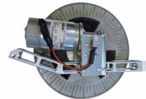
Winch unit for Scheibe Falke SF 25
