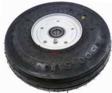
Red Dot marking on larger aircraft tires
