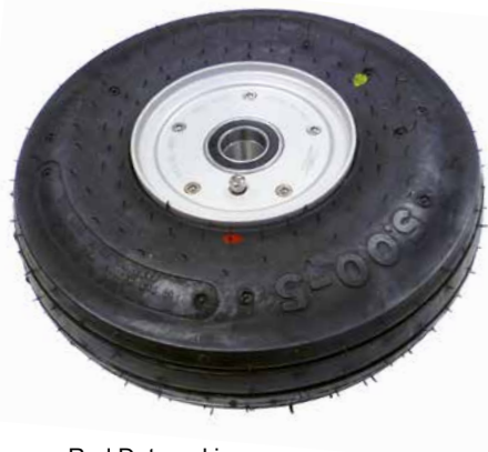
Red Dot marking on larger aircraft tires
