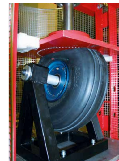
Static load test of a complete wheel
