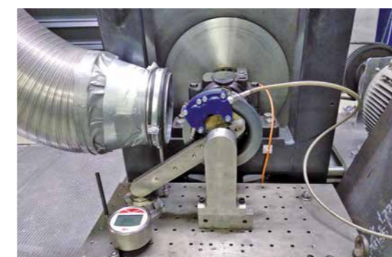
Brake test with flywheel to determine braking performance
