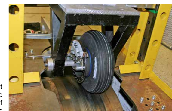
Brake test with flywheel to determine braking performance
