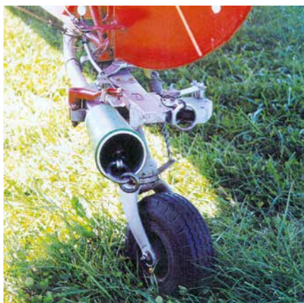
CRG in PA 25 with parallel use of tow release E 85
