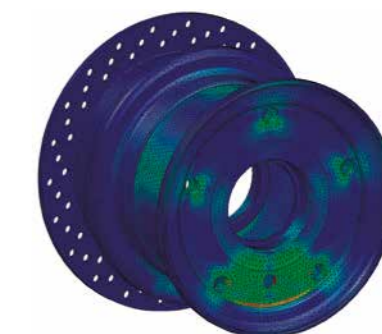
FEM-based analysis of Penta disk brake wheel
